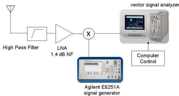
Figure 2: System setup diagram at receiver side.
