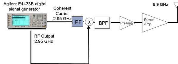
Figure 1: System setup diagram at transmitter side.
