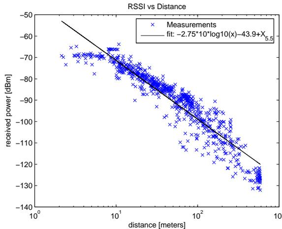
Figure 3: Pathloss measurements and the log-normal model fit.
