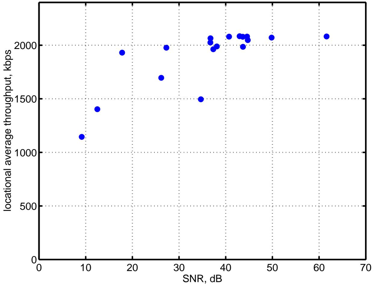
Figure 5.5: All measurements averaged for all directions at each measurement location for Scenario A, 3Com System
