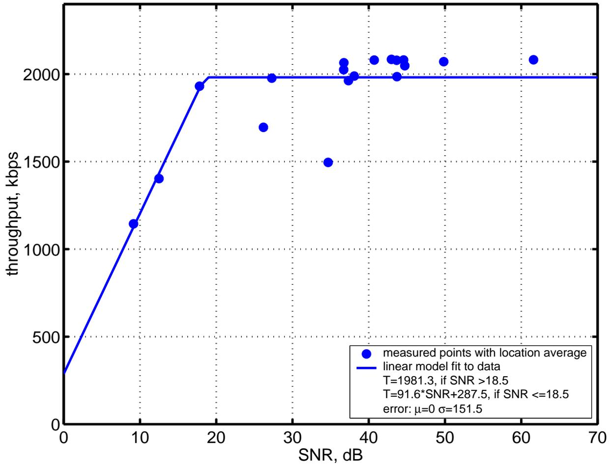
Figure 6.2: 3Com Scenario A, Location Averaged Data and Linear Throughput Prediction Model
