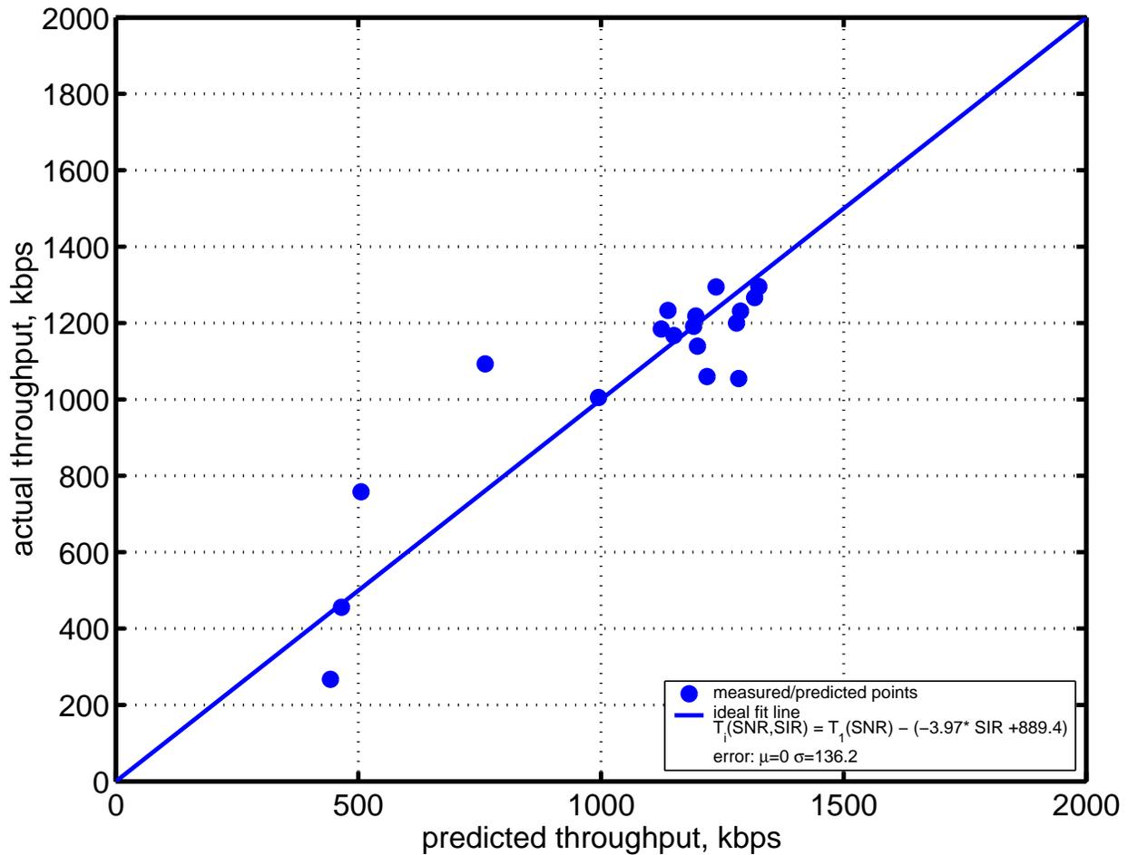
Figure 6.14: 3Com Scenario C, One User with Interference, throughput prediction model. This figure shows the predicted versus actual throughput results and an ideal fit line
