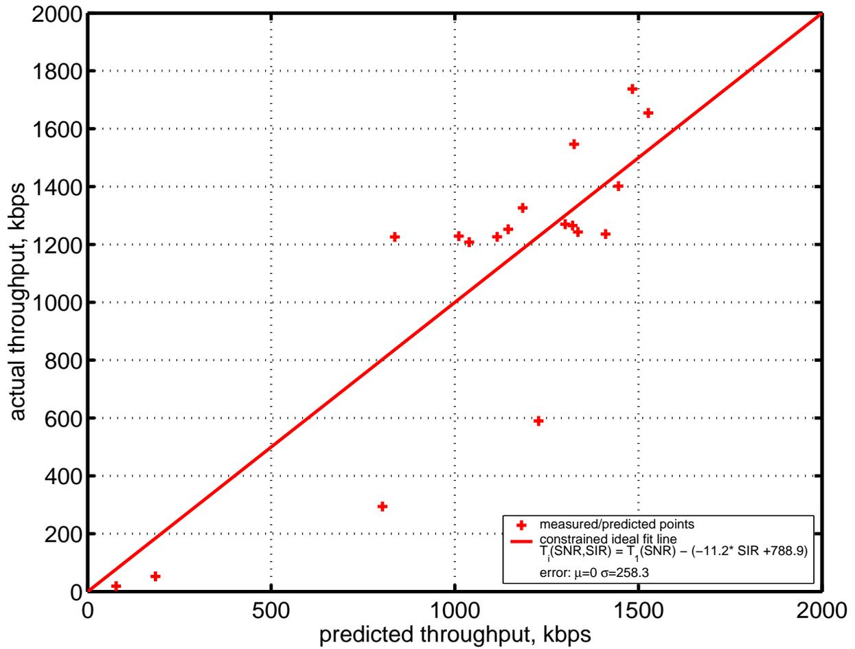
Figure 6.15: Constrained WaveLAN Scenario C, One User with Interference, throughput prediction Model. This figure shows the predicted versus actual throughput results and an ideal fit line
