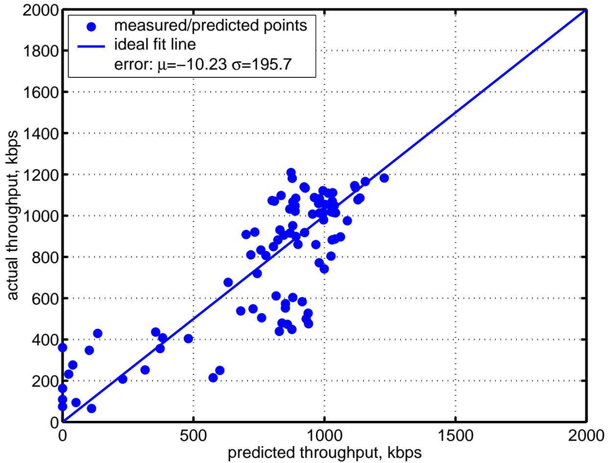
Figure 6.20: 3Com Scenario D, Constrained 2 User with Interference, throughput prediction model. This figure shows the predicted versus actual throughput results and an ideal fit line
