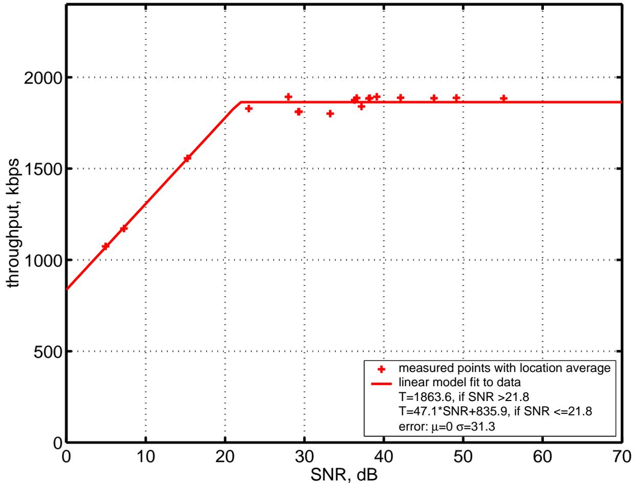
Figure 6.1: WaveLAN Scenario A, Location Averaged Data and Linear Throughput Prediction Model
