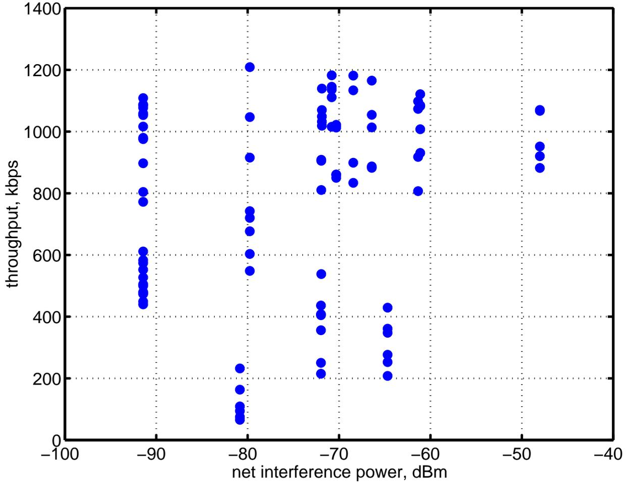
Figure 5.33: Plots of the 3Com measured throughput versus the calculated net interference power averaged over all cardinal directions for each physical location. All data points for both clients are shown in the graph.
