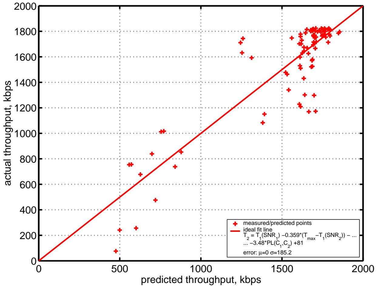
Figure 6.9: WaveLAN Scenario B, 2 User Prediction Model. This figure shows the predicted versus actual throughput results and an ideal fit line
