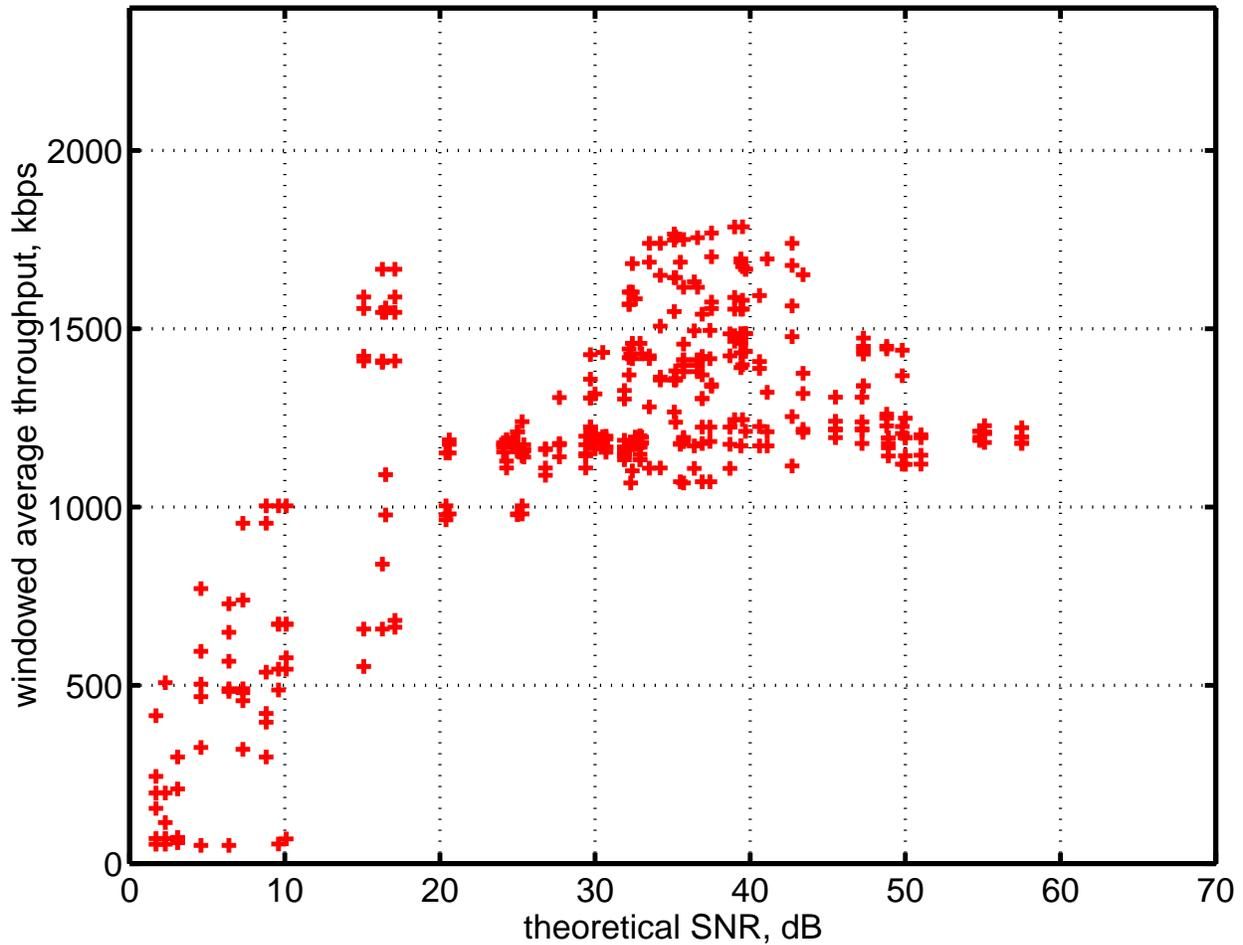
Figure 5.21: All measurements averaged over similar signal strength (i.e. RSSI) locations for Scenario D, WaveLAN System
