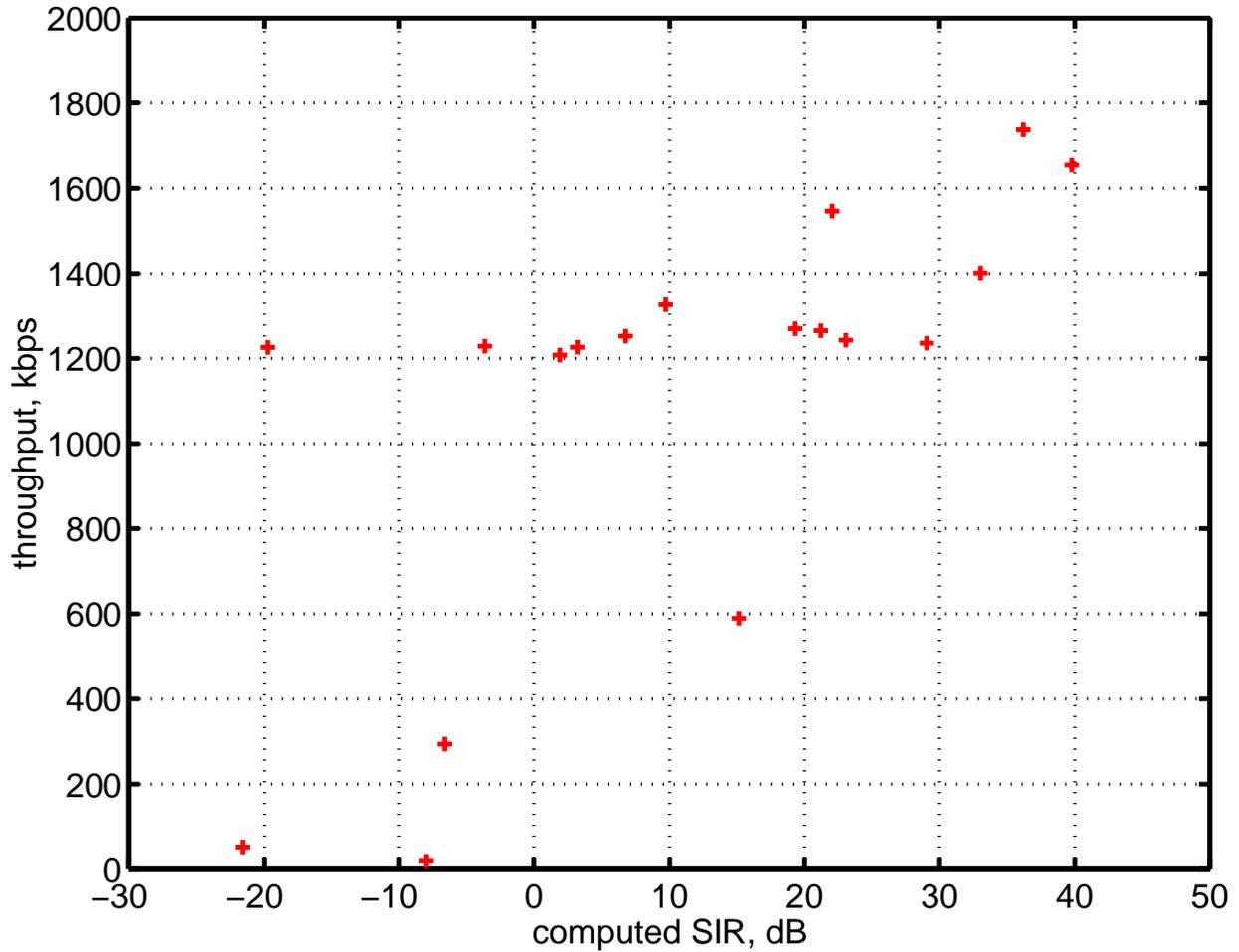
Figure 5.28: Plots of the WaveLAN measured throughput versus the calculated SIR averaged over all cardinal directions for each physical location
