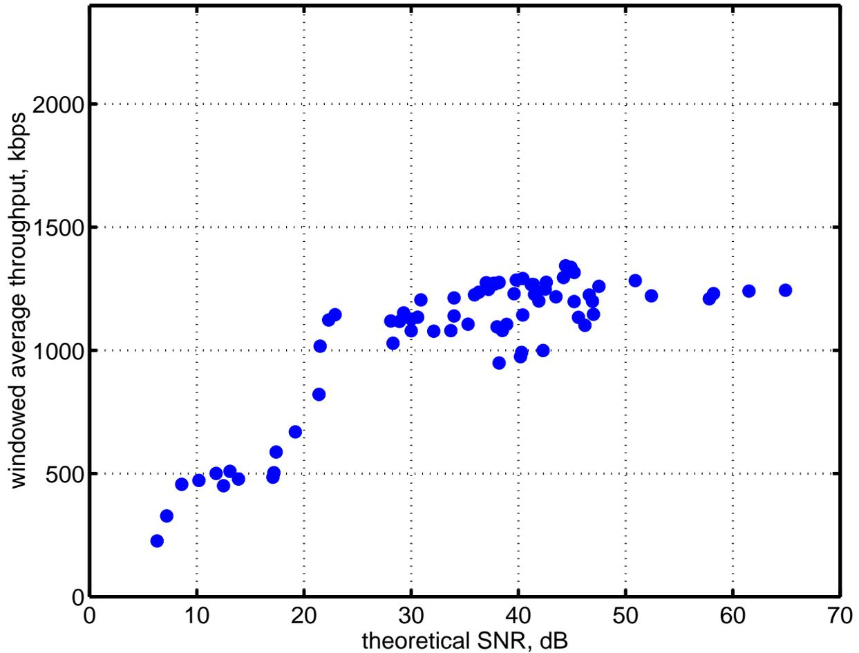
Figure 5.18: All measurements averaged over similar signal strength (i.e. RSSI) locations for Scenario C, 3Com System
