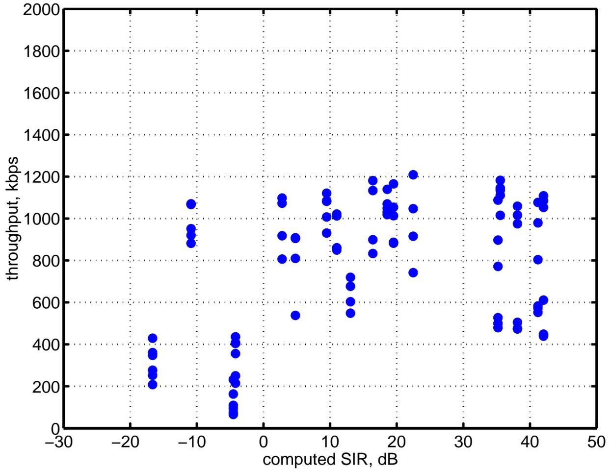
Figure 5.34: Plots of the 3Com measured throughput versus the calculated SIR averaged over all cardinal directions for each physical location. All data points for both clients are shown in the graph.
