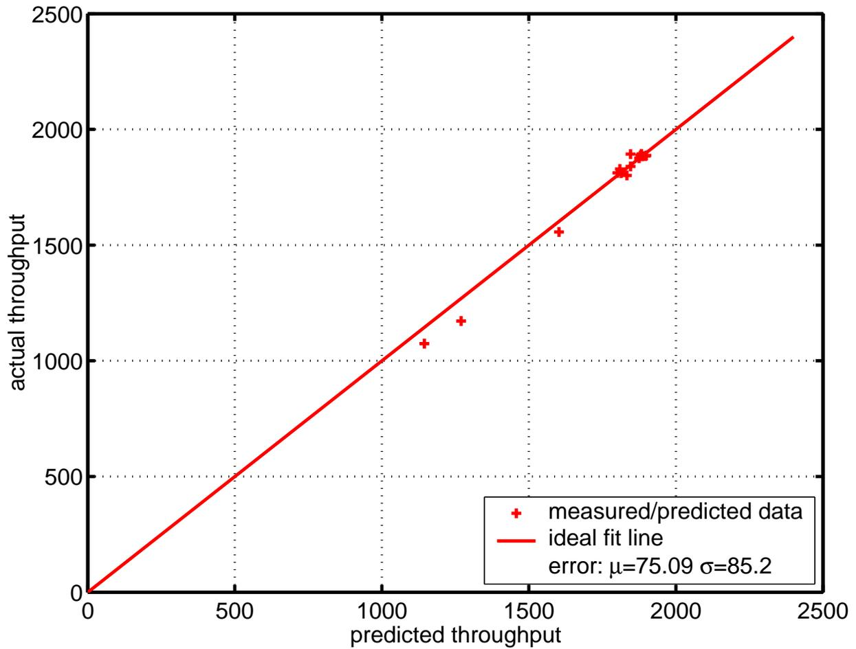
Figure 7.1: Comparison of the fit for Scenario A when throughput is predicted directly from a model of the building environment for the WaveLAN network.
