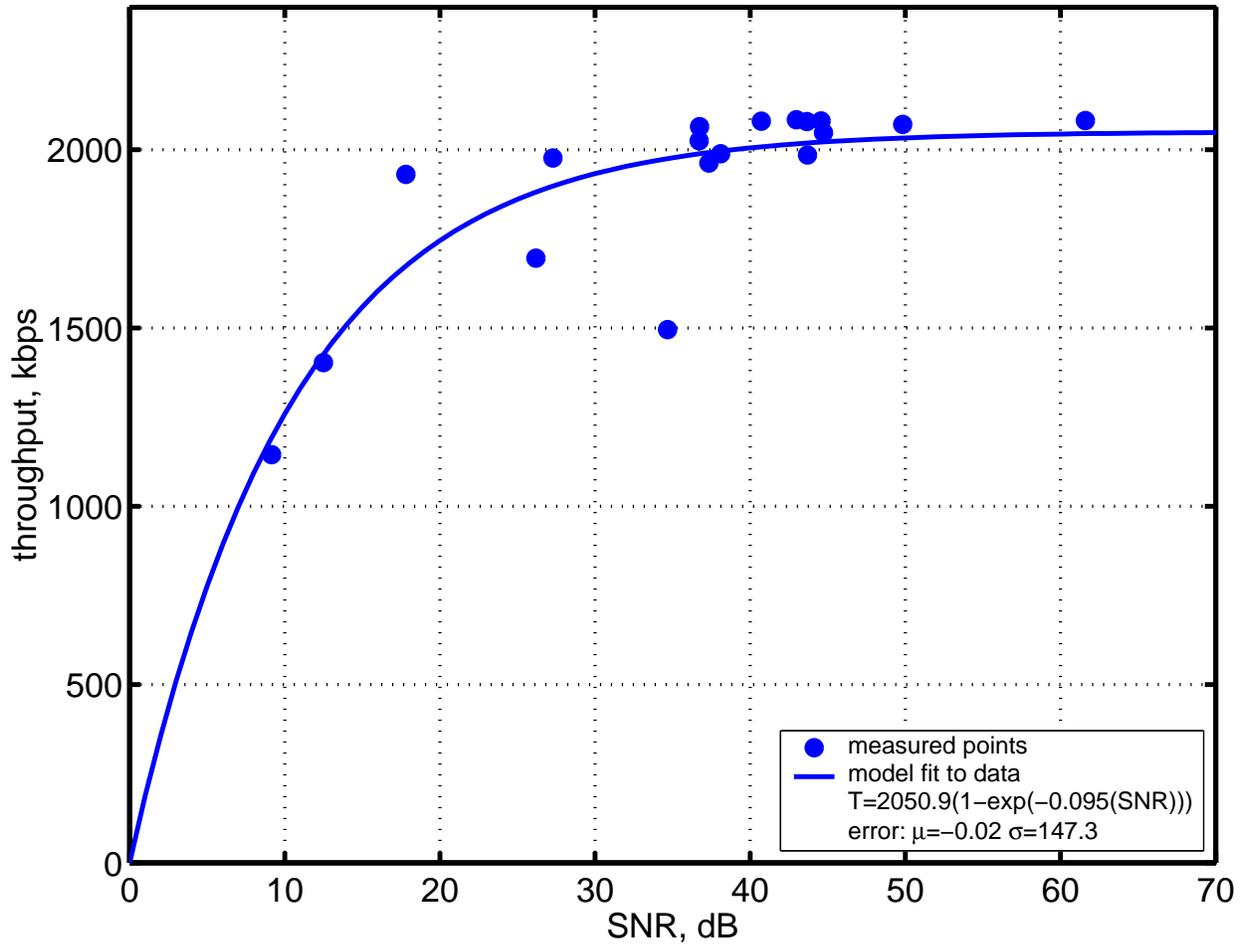
Figure 6.8: 3Com Scenario A, Location Averaged Data and Exponential Constrained Throughput Prediction Model
