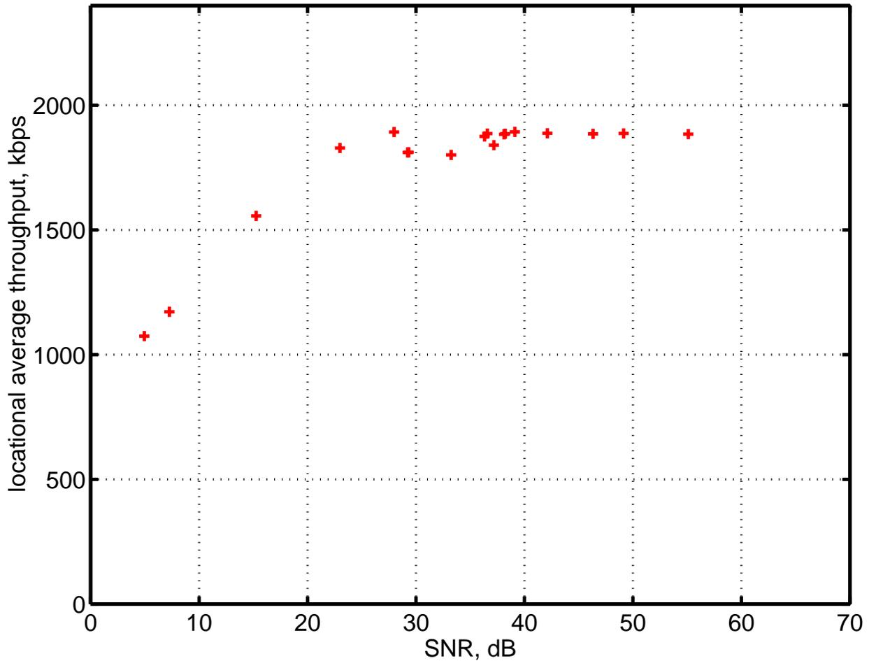
Figure 5.2: All measurements averaged for all directions at each measurement location for Scenario A, WaveLAN System
