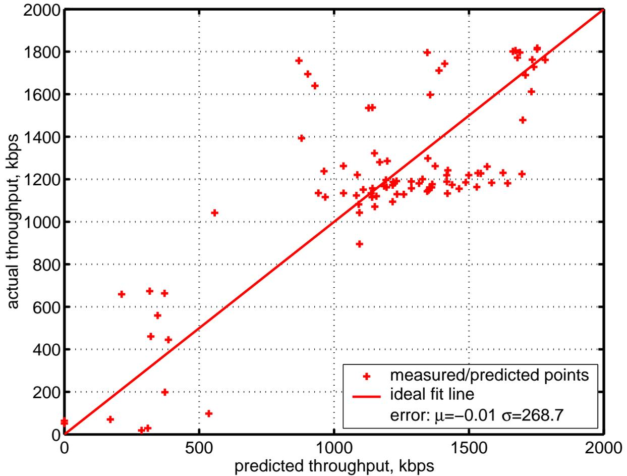
Figure 6.17: WaveLAN Scenario D, 2 User with Interference, throughput prediction Model. This figure shows the predicted versus actual throughput results and an ideal fit line
