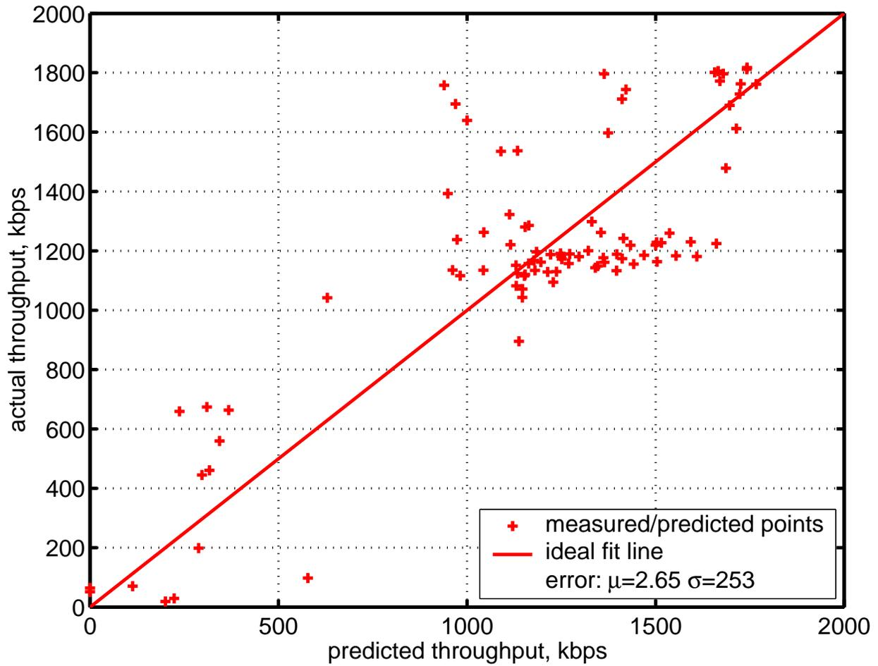
Figure 6.19: WaveLAN Scenario D, Constrained 2 User with Interference, throughput prediction Model. This figure shows the predicted versus actual throughput results and an ideal fit line
