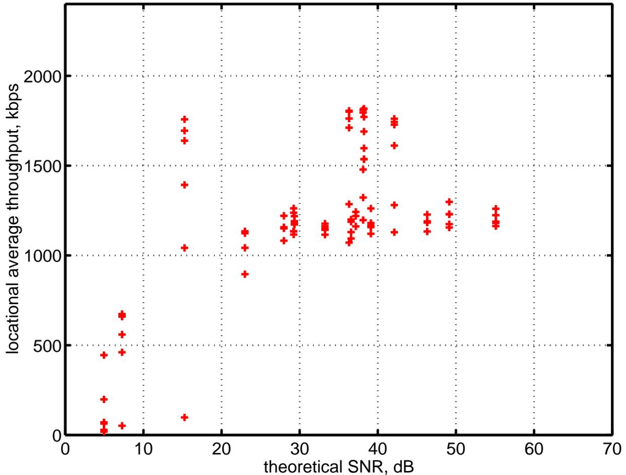
Figure 5.20: All measurements averaged for all directions at each measurement location for Scenario D, WaveLAN System
