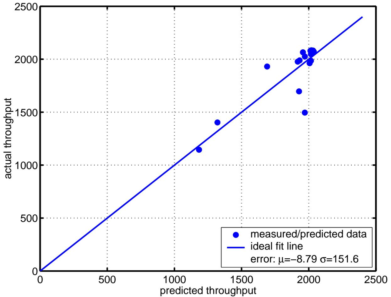
Figure 7.2: Comparison of the fit for Scenario A when throughput is predicted directly from a model of the building environment for the 3Com network.
