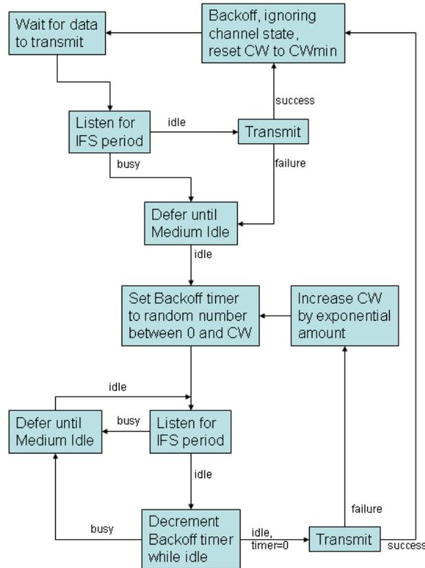
Figure A.9: Flow chart of the process of sending data packets under the CSMA/CA based Distributed Coordination Function (DCF). Created using information in [30].
