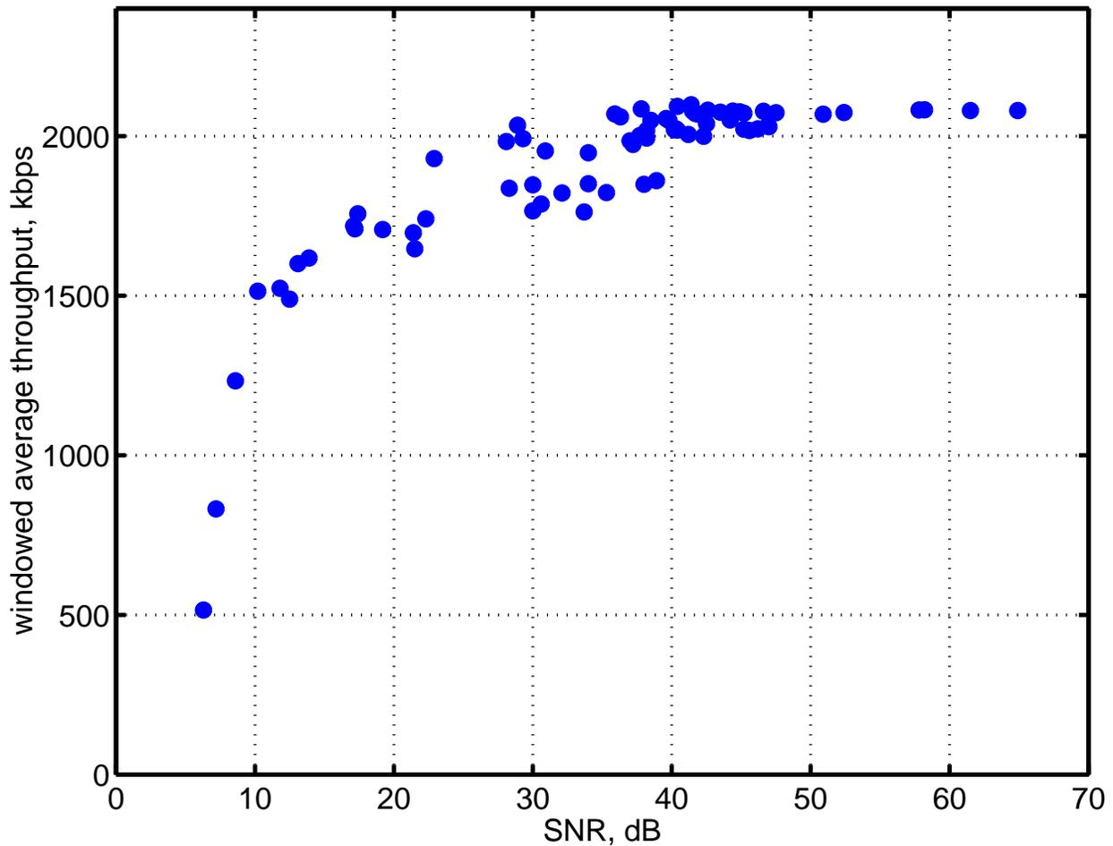
Figure 5.6: All measurements averaged over similar signal strength (i.e. RSSI) locations for Scenario A, 3Com System
