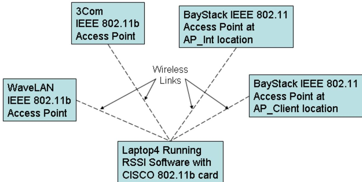
Figure 4.2: Logical layout diagram of the RSSI measurement hardware configurations
