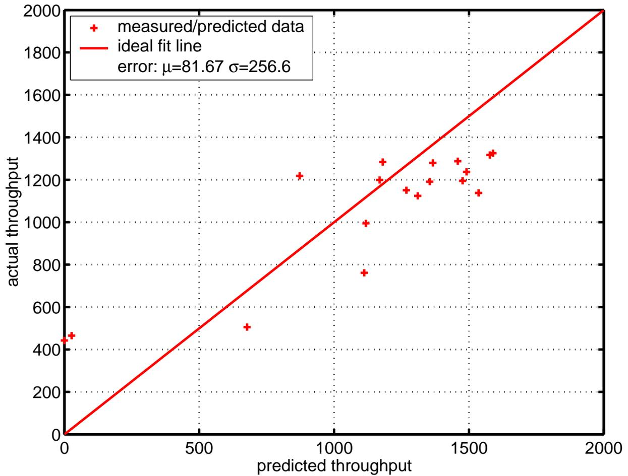
Figure 7.5: Comparison of the fit for Scenario C when throughput is predicted directly from a model of the building environment for the WaveLAN network.
