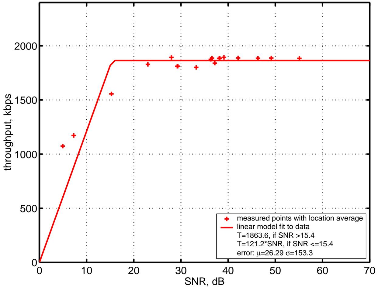
Figure 6.3: WaveLAN Scenario A, Location Averaged Data and Linear Constrained Throughput Prediction Model
