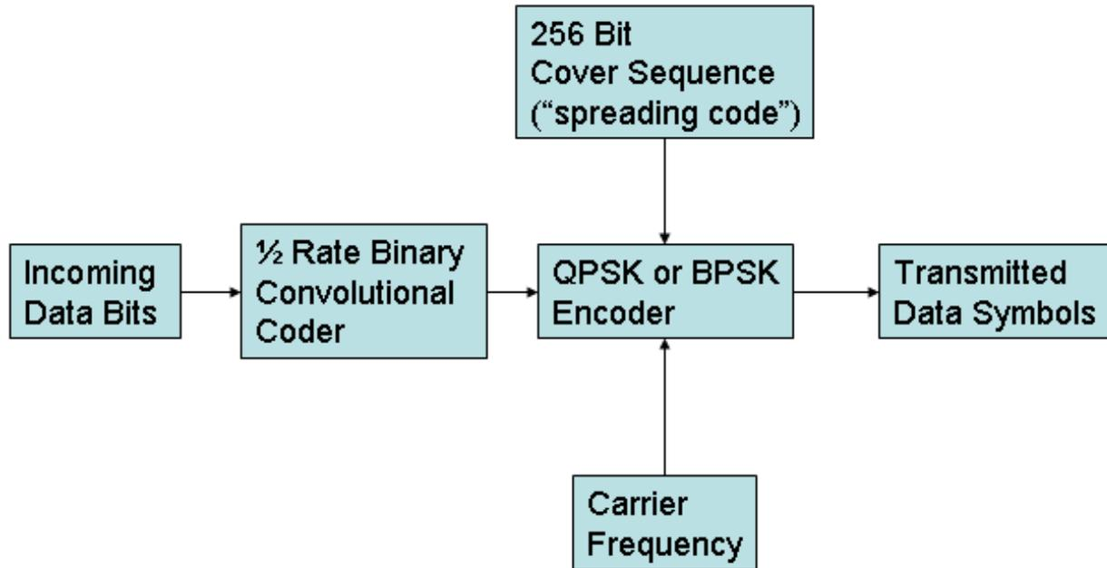
Figure A.6: A block diagram of the PBCC encoding technique. Created using information from [31].
