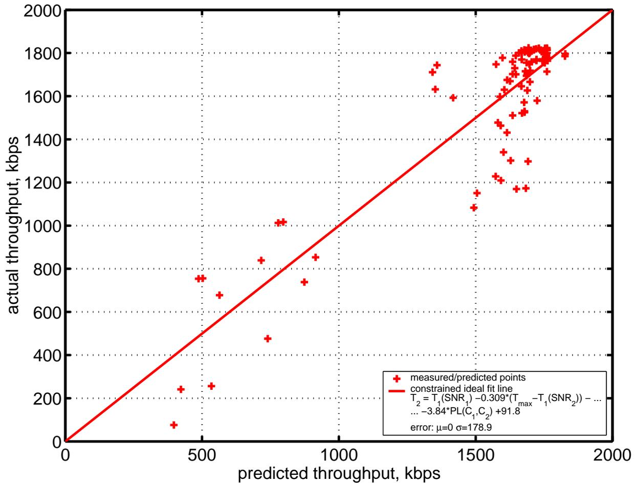
Figure 6.11: WaveLAN Scenario B, 2 User Constrained Prediction Model. This figure shows the predicted versus actual throughput results and an ideal fit line
