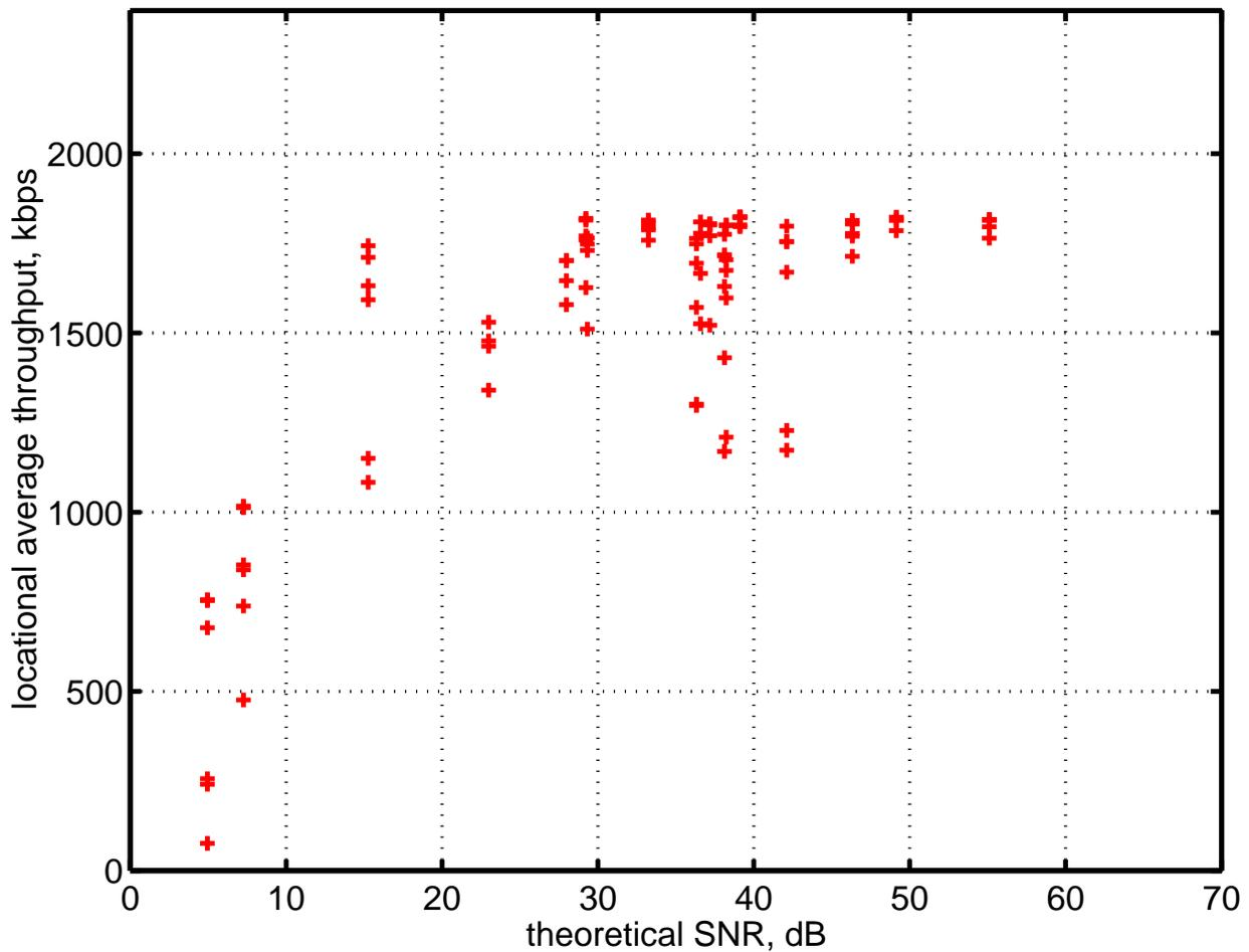
Figure 5.8: All measurements averaged for all directions at each measurement location for Scenario B, WaveLAN System
