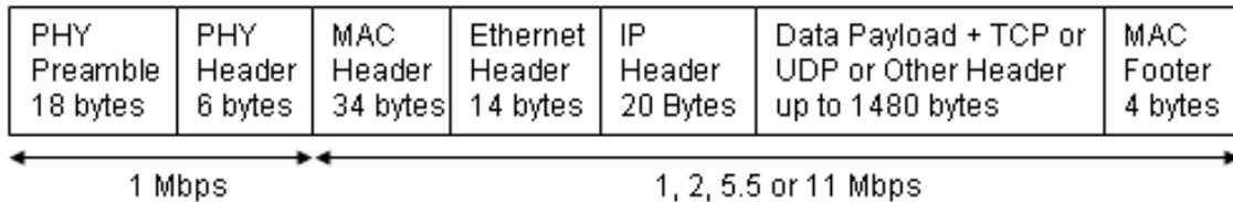
Figure A.7: Basic structure of the IEEE 802.11b packet as it's transmitted on the physical layer is shown here. Adapted from [31].
