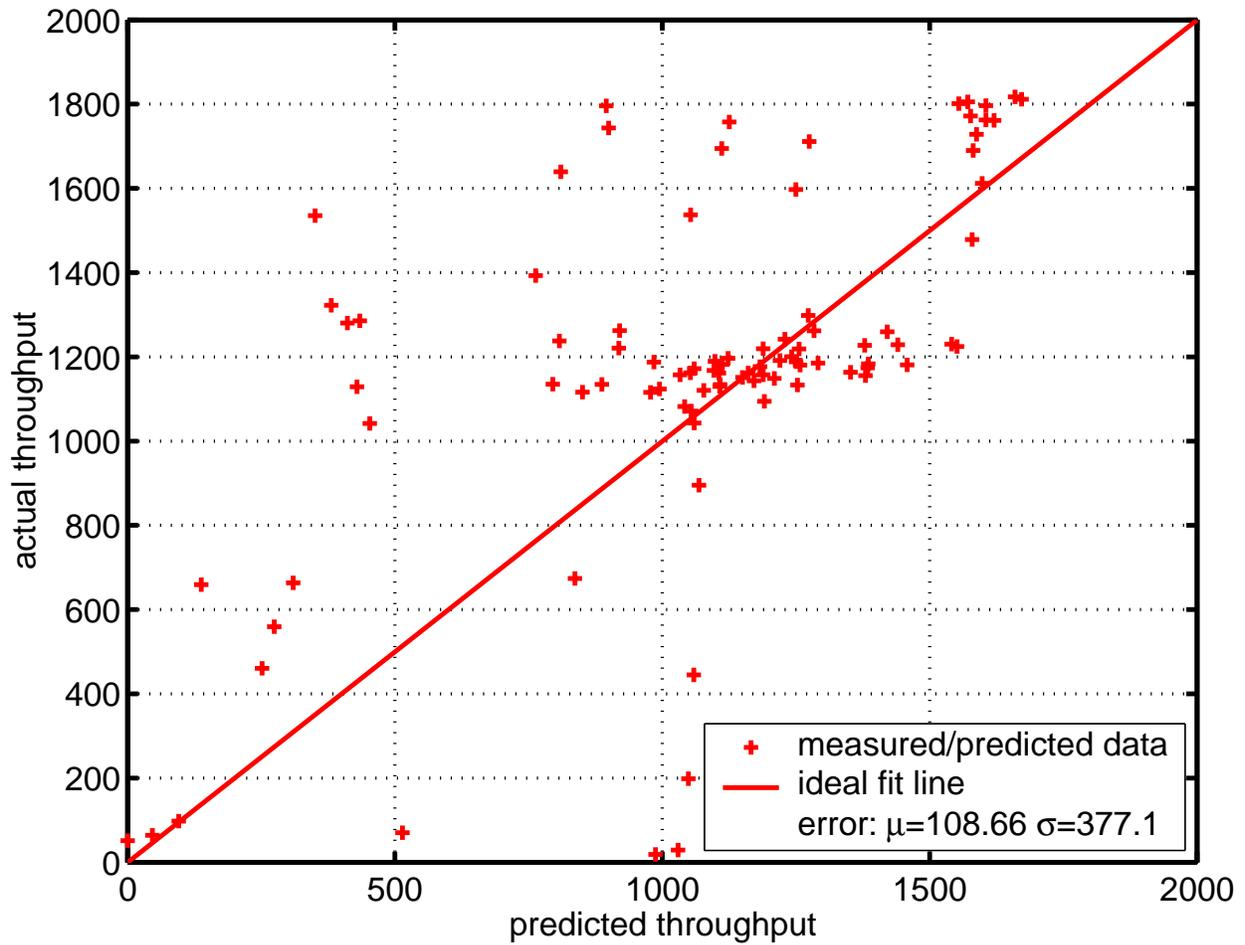
Figure 7.7: Comparison of the fit for Scenario D when throughput is predicted directly from a model of the building environment for the WaveLAN network.
