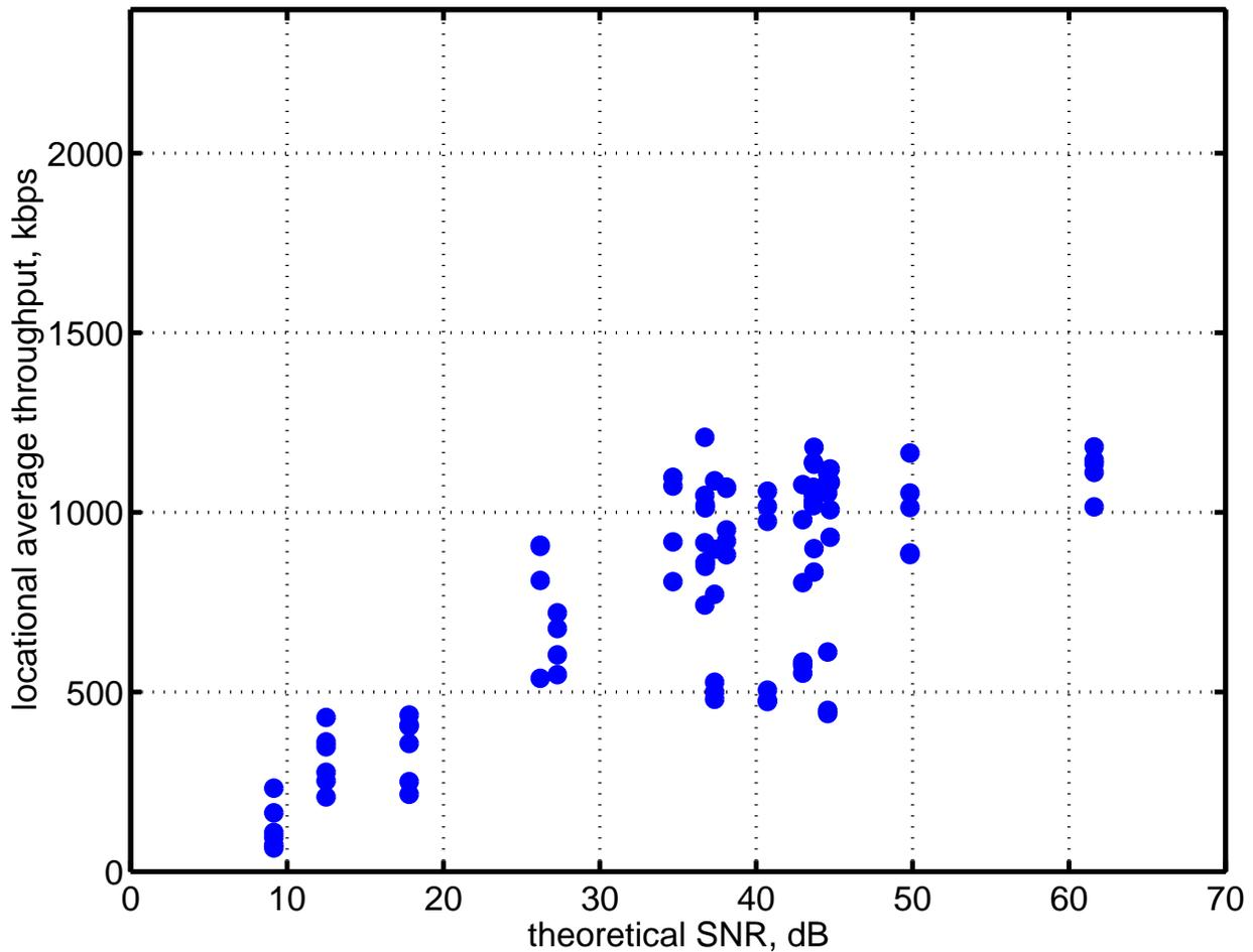
Figure 5.23: All measurements averaged for all directions at each measurement location for Scenario D, 3Com System
