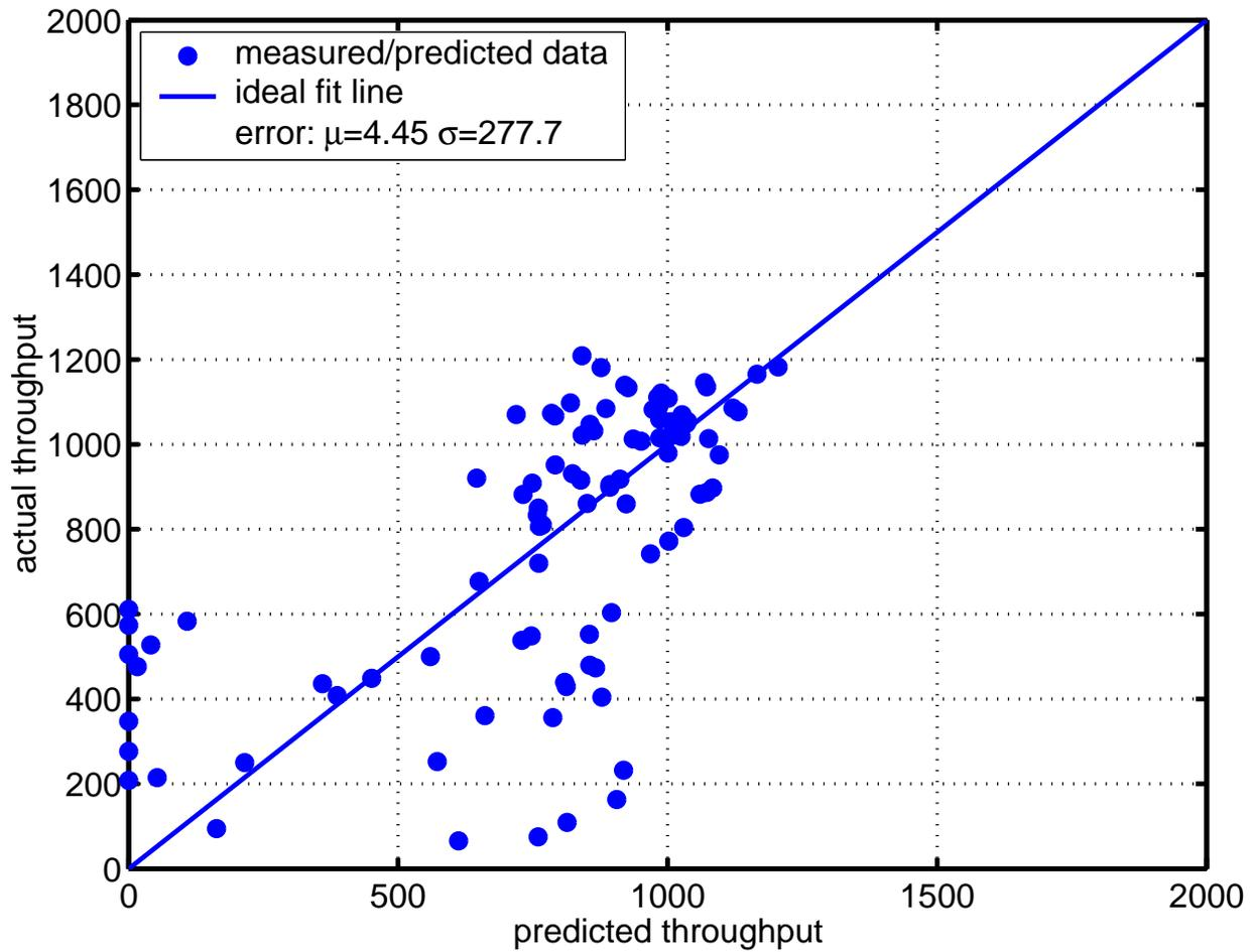
Figure 7.8: Comparison of the fit for Scenario D when throughput is predicted directly from a model of the building environment for the 3Com network.
