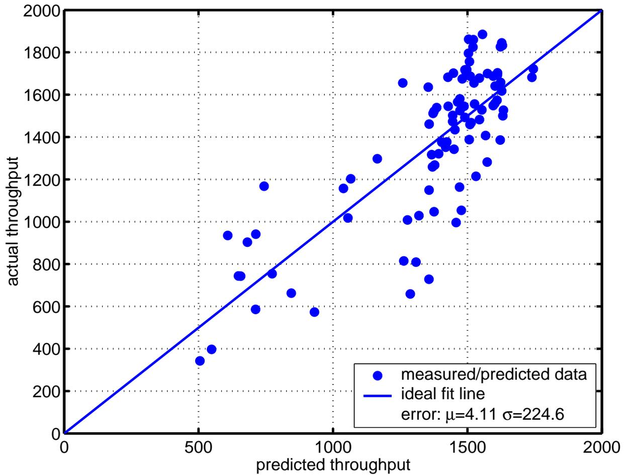
Figure 7.4: Comparison of the fit for Scenario B when throughput is predicted directly from a model of the building environment for the 3Com network.
