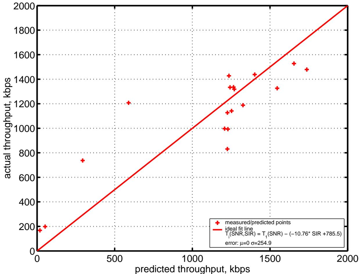
Figure 6.13: WaveLAN Scenario C, One User with Interference, throughput prediction Model. This figure shows the predicted versus actual throughput results and an ideal fit line
