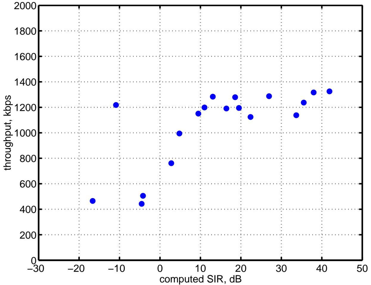
Figure 5.30: Plots of the 3Com measured throughput versus the calculated SIR averaged over all cardinal directions for each physical location
