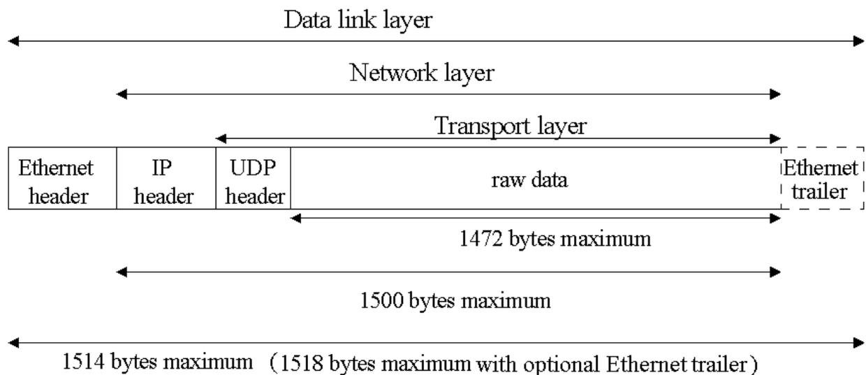
Figure 3.4: Format of LANFielder Test Packet
