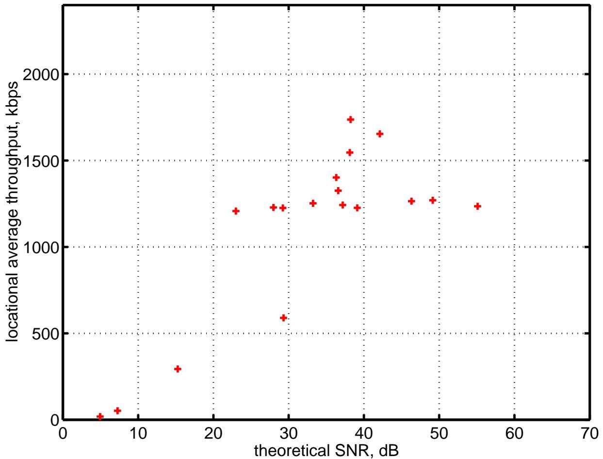
Figure 5.14: All measurements averaged for all directions at each measurement location for Scenario C, WaveLAN System
