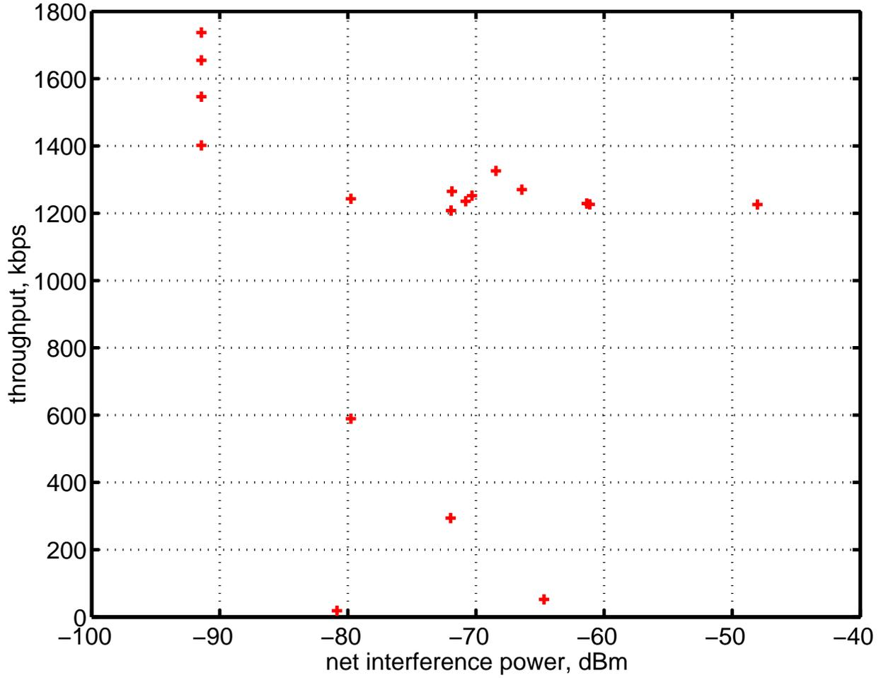
Figure 5.27: Plots of the WaveLAN measured throughput versus the calculated net interference power averaged over all cardinal directions for each physical location
