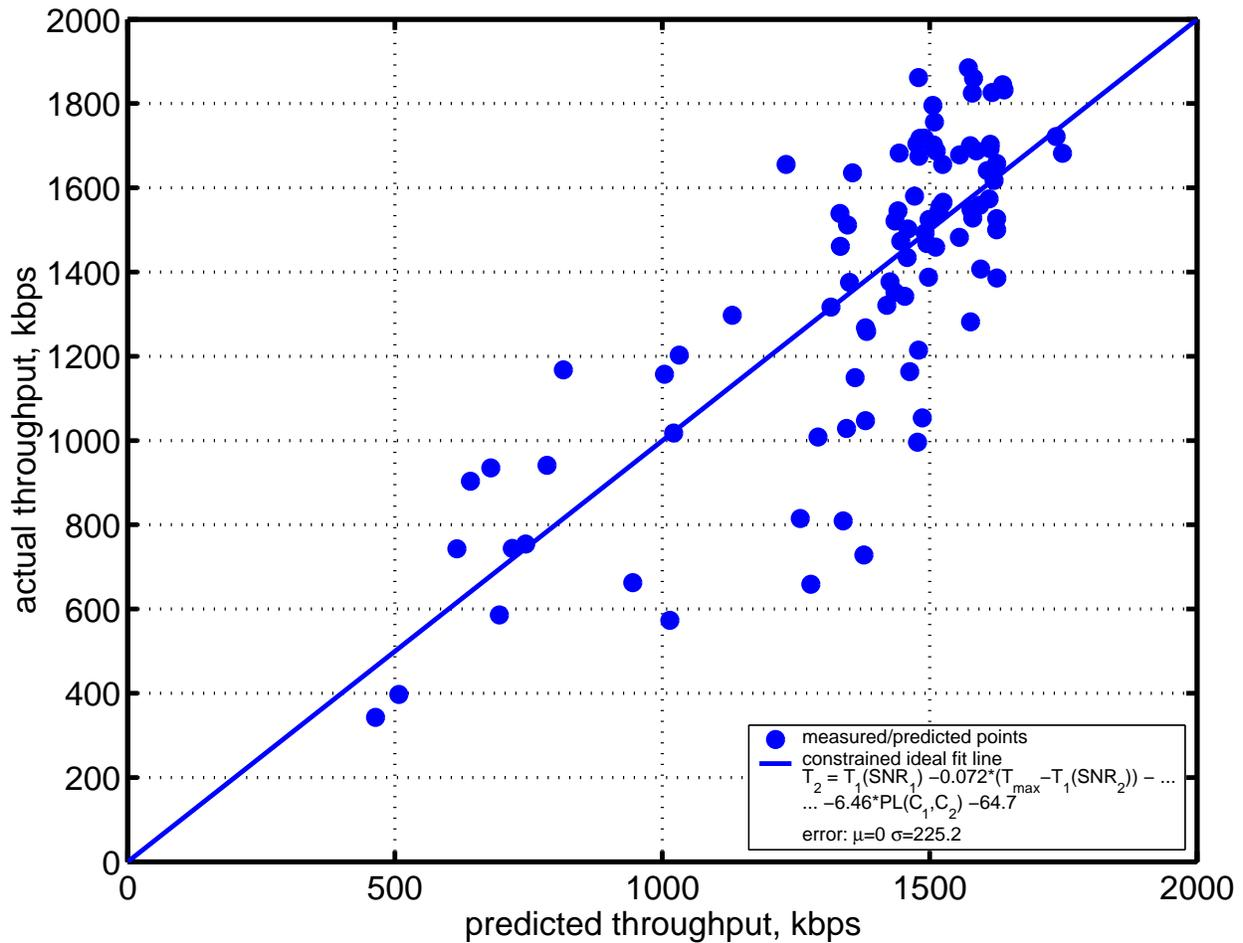
Figure 6.12: 3Com Scenario B, 2 User Constrained Prediction Model. This figure shows the predicted versus actual throughput results and an ideal fit line
