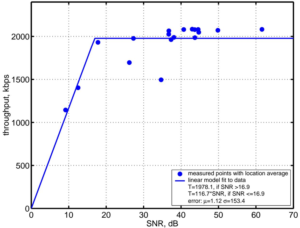
Figure 6.4: 3Com Scenario A, Location Averaged Data and Linear Constrained Throughput Prediction Model
