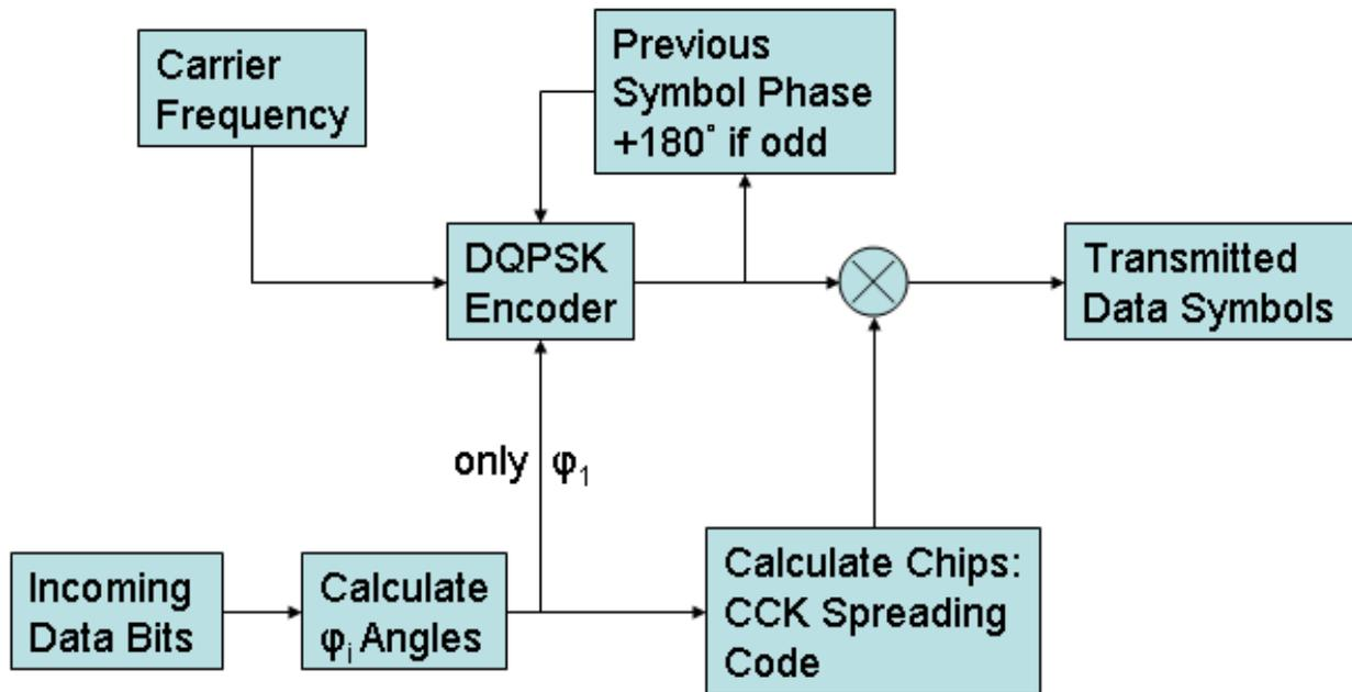
Figure A.5: Conceptual block diagram of the CCK encoding process carried out by the transmitter. Created using information from [31].
