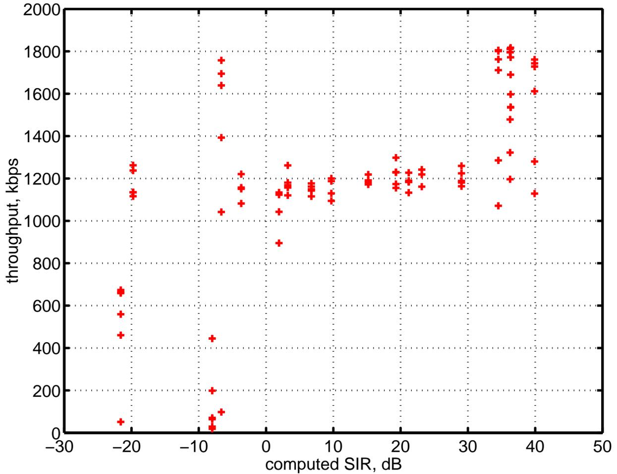
Figure 5.32: Plots of the WaveLAN measured throughput versus the calculated SIR averaged over all cardinal directions for each physical location. All data points for both clients are shown in the graph.
