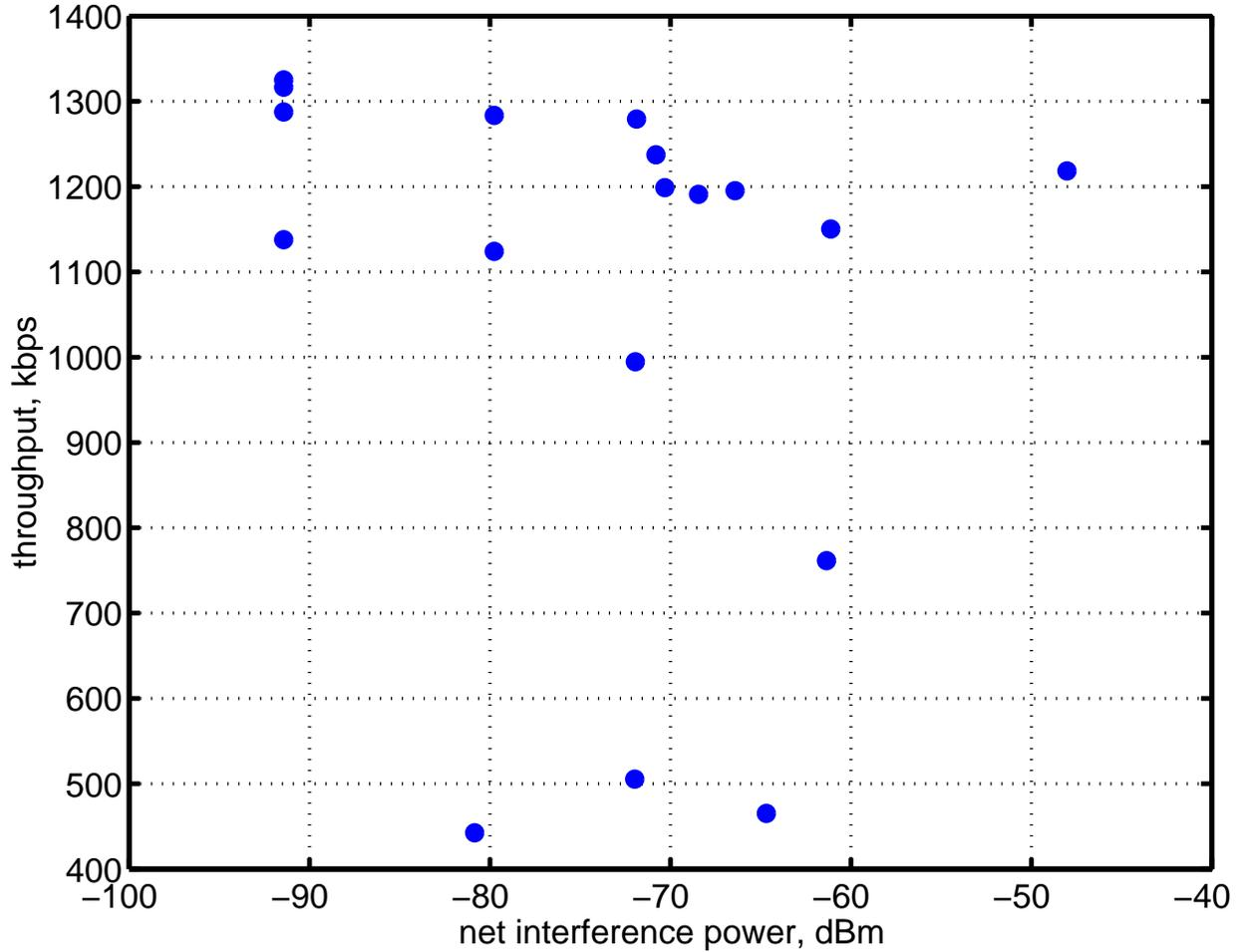
Figure 5.29: Plots of the 3Com measured throughput versus the calculated net interference power averaged over all cardinal directions for each physical location
