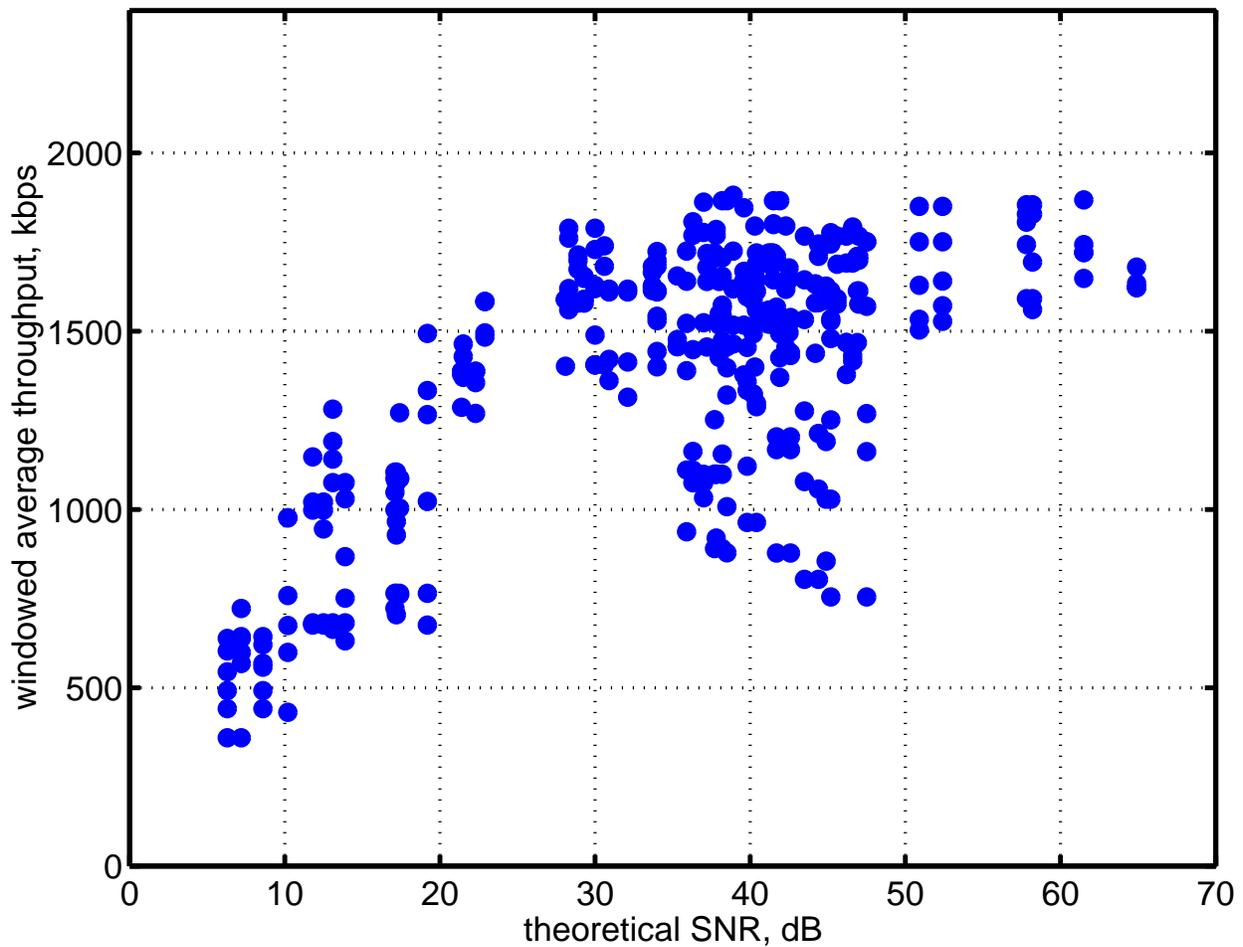
Figure 5.12: All measurements averaged over similar signal strength (i.e. RSSI) locations for Scenario B, 3Com System
