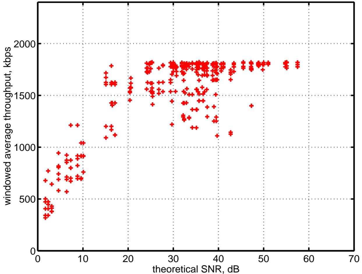
Figure 5.9: All measurements averaged over similar signal strength (i.e. RSSI) locations for Scenario B, WaveLAN System
