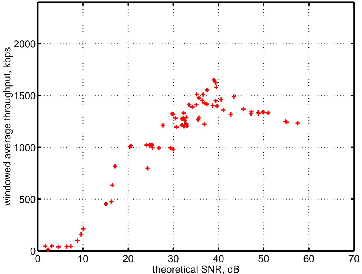
Figure 5.15: All measurements averaged over similar signal strength (i.e. RSSI) locations for Scenario C, WaveLAN System
