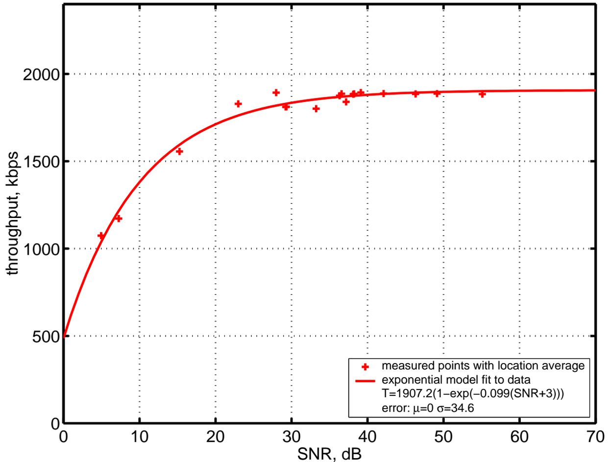
Figure 6.5: WaveLAN Scenario A, Location Averaged Data and Exponential Throughput Prediction Model
