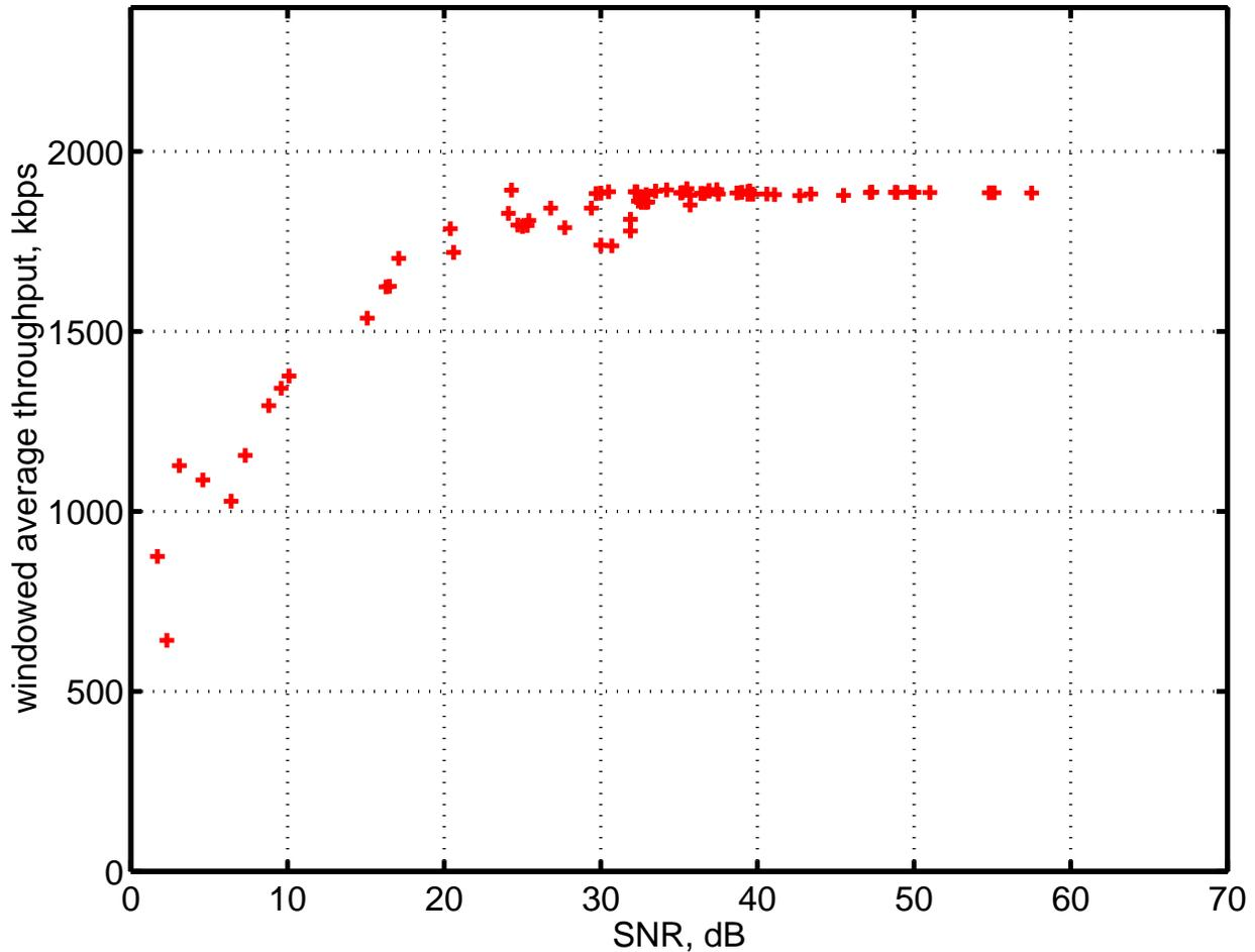
Figure 5.3: All measurements averaged over similar signal strength (i.e. RSSI) locations for Scenario A, WaveLAN System
