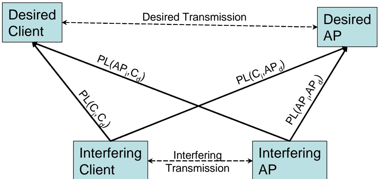
Figure 5.26: A diagram of the interference paths between the different wireless LAN users in Scenarios C and D.
