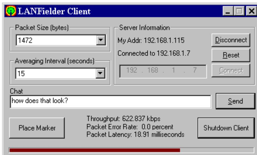
Figure 3.2: A LANFielder Client in operation
