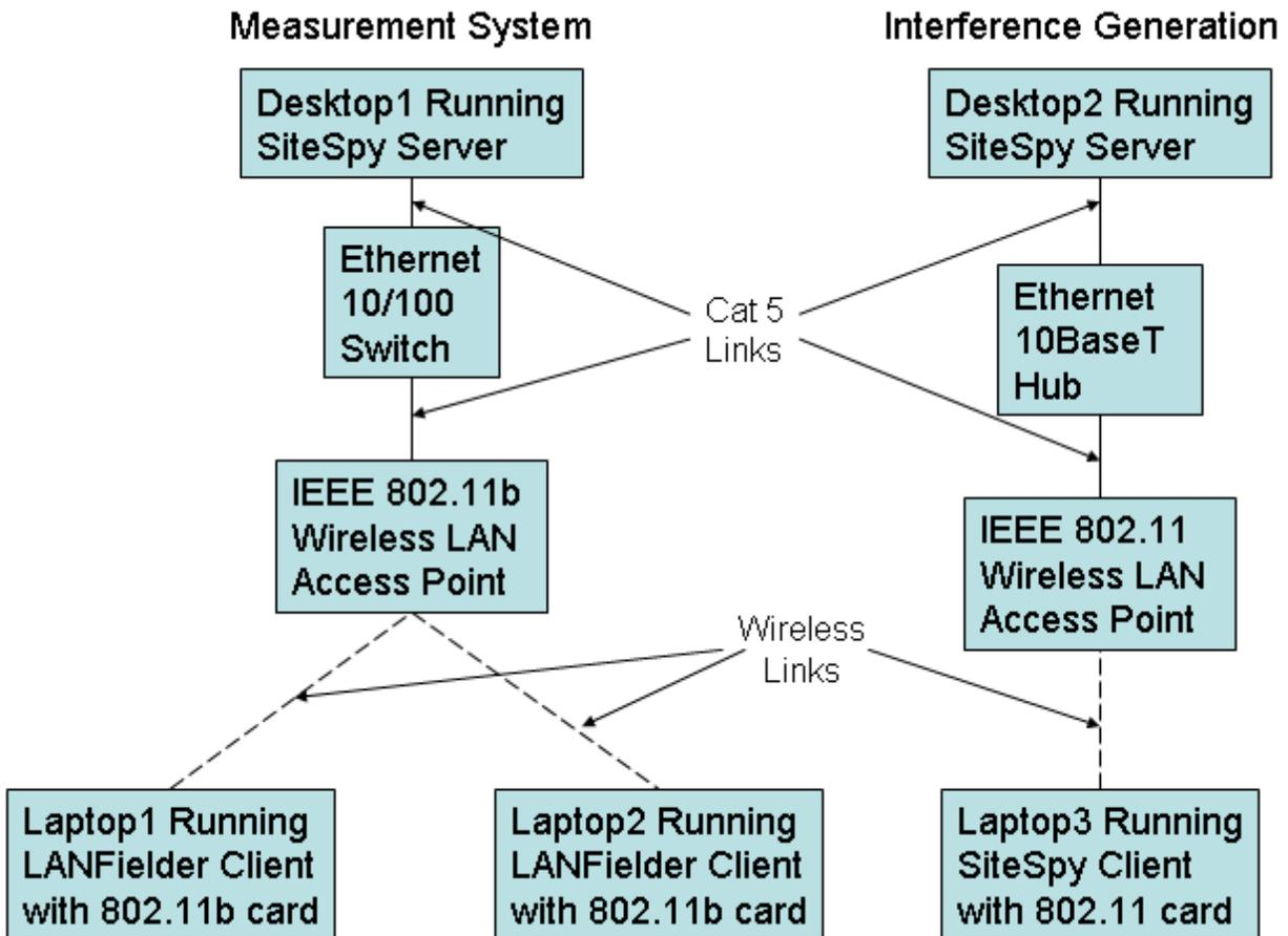
Figure 4.1: Logical layout of measurements and the software used.
