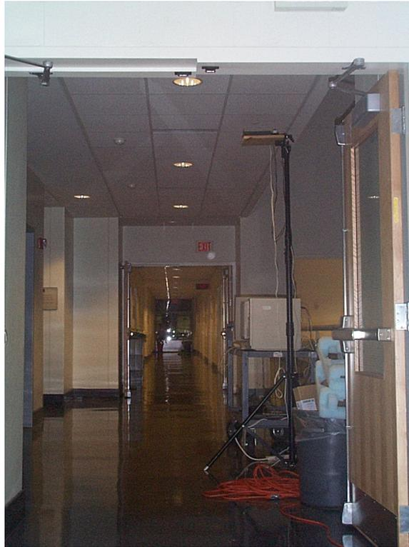
Figure 4.7: A picture of the wireless LAN access point transmitter location for Case II
