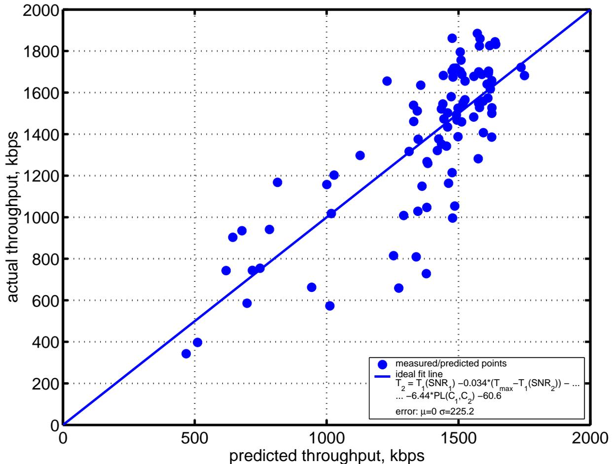
Figure 6.10: 3Com Scenario B, 2 User Prediction Model. This figure shows the predicted versus actual throughput results and an ideal fit line
