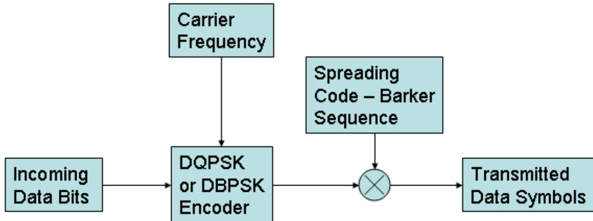
Figure A.4: Illustration of the basic IEEE 802.11 Spreading technique. Created using information from [30] and [31].
