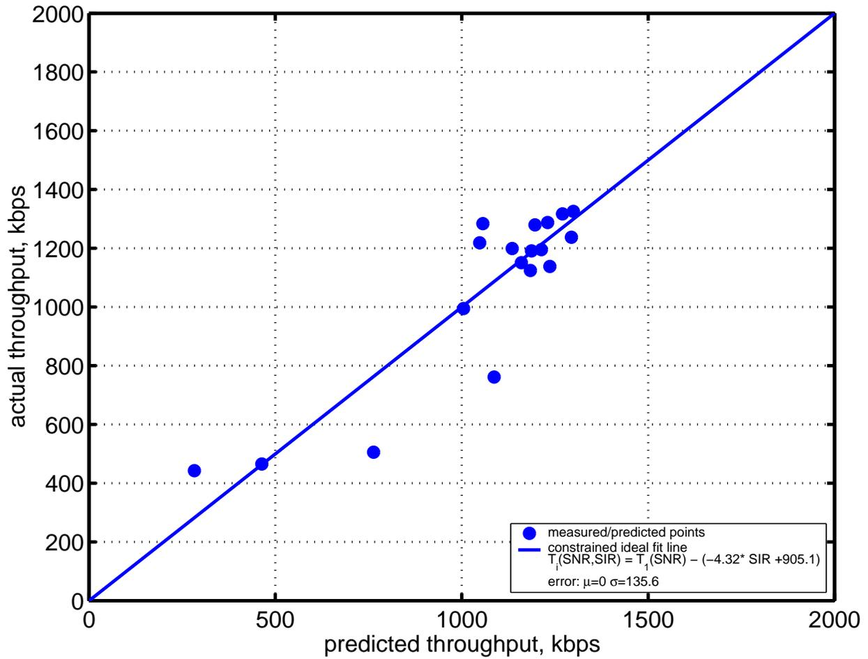
Figure 6.16: Constrained 3Com Scenario C, One User with Interference, throughput prediction model. This figure shows the predicted versus actual throughput results and an ideal fit line
