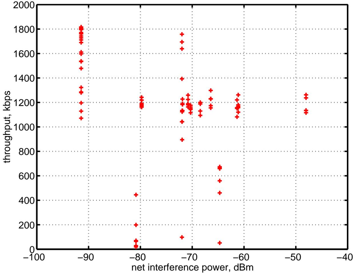
Figure 5.31: Plots of the WaveLAN measured throughput versus the calculated net interference power averaged over all cardinal directions for each physical location. All data points for both clients are shown in the graph.
