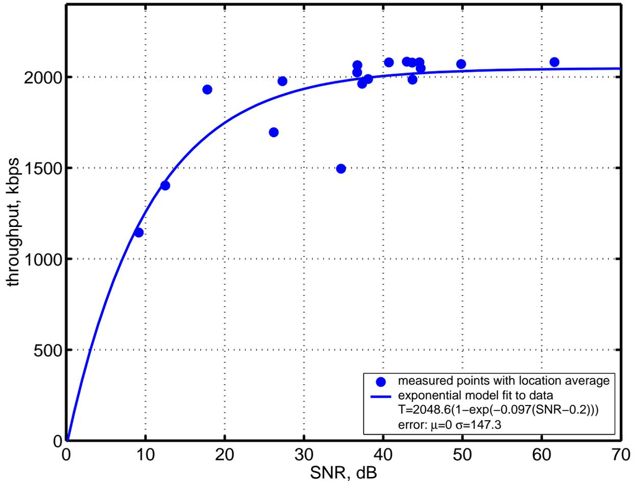
Figure 6.6: 3Com Scenario A, Location Averaged Data and Exponential Throughput Prediction Model
