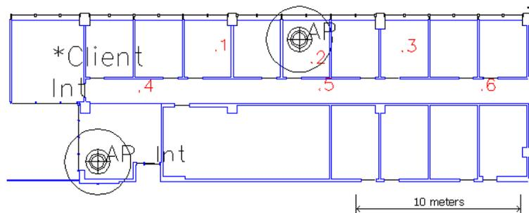
Figure 4.9: Physical Layout of Measurement Equipment in Case III
