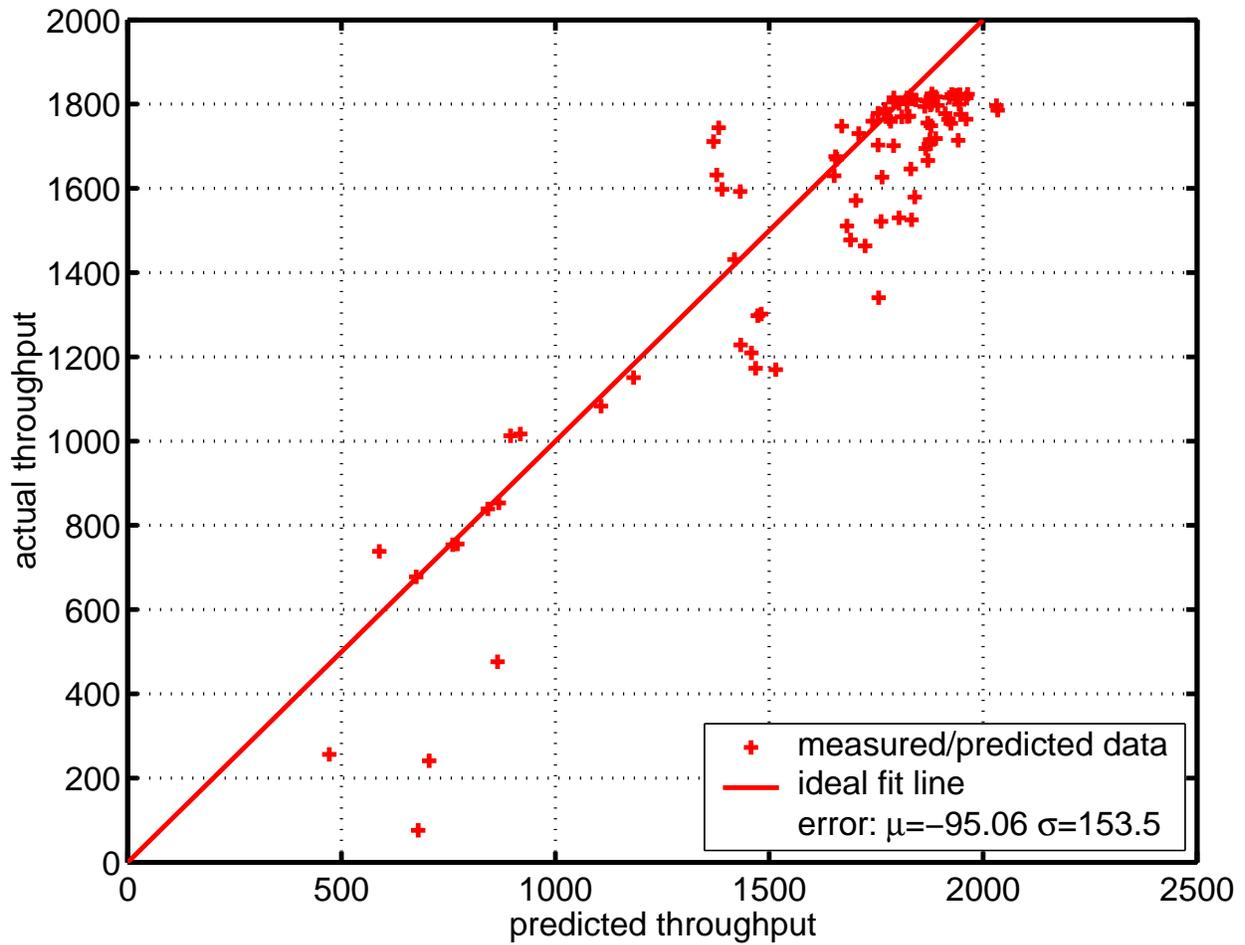
Figure 7.3: Comparison of the fit for Scenario B when throughput is predicted directly from a model of the building environment for the WaveLAN network.
