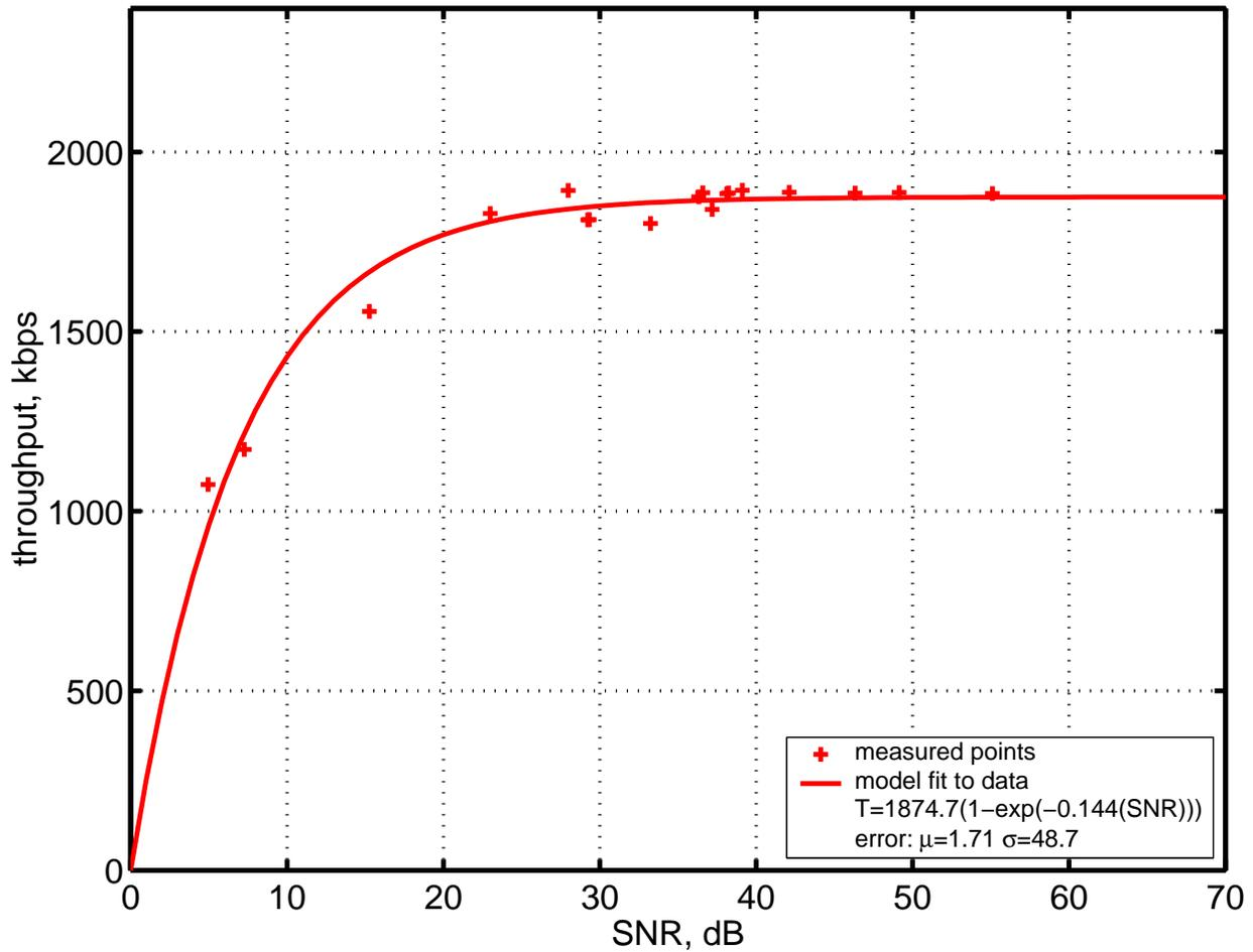
Figure 6.7: WaveLAN Scenario A, Location Averaged Data and Exponential Constrained Throughput Prediction Model
