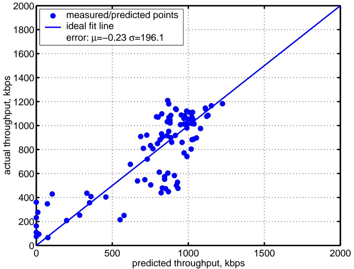
Figure 6.18: 3Com Scenario D, 2 User with Interference, throughput prediction model. This figure shows the predicted versus actual throughput results and an ideal fit line
