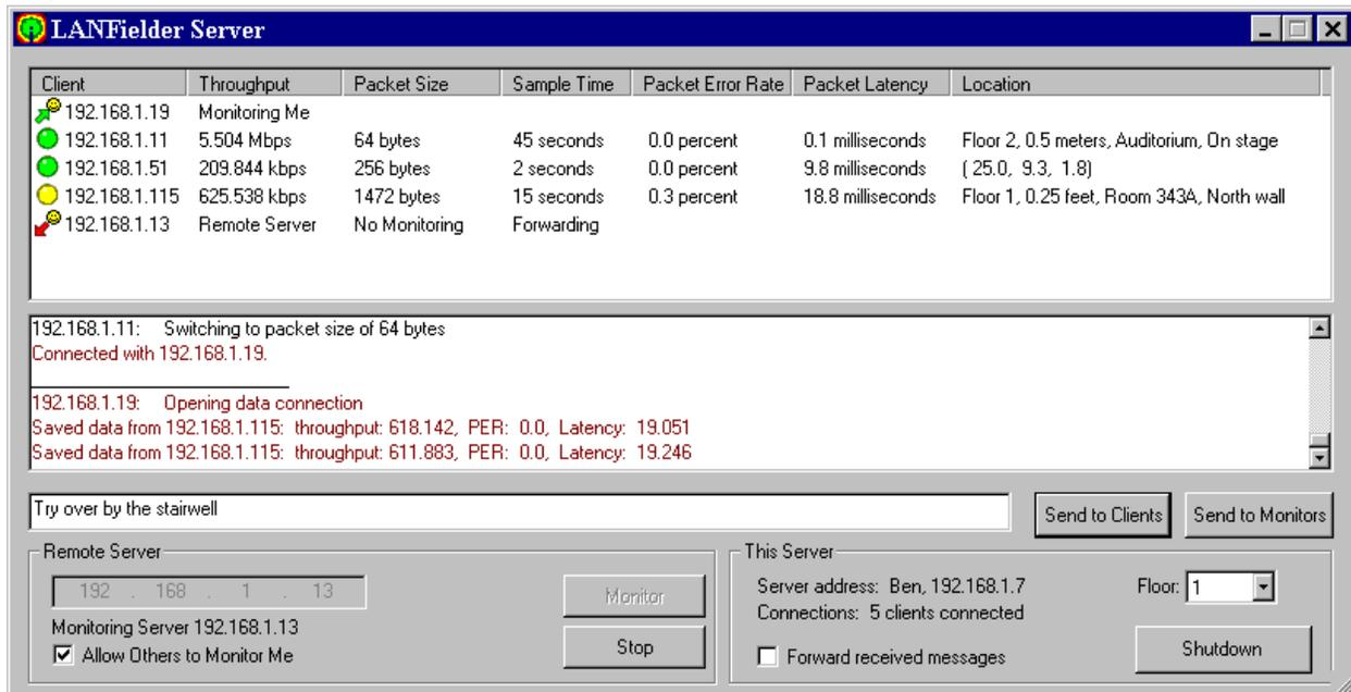
Figure 3.3: A LANFielder Server with several clients connected.
