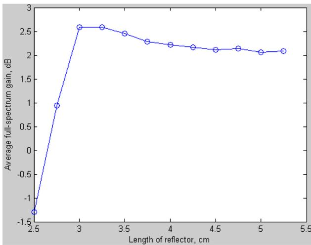
Fig. 6. Results of Reflector Length Variation Experiment
