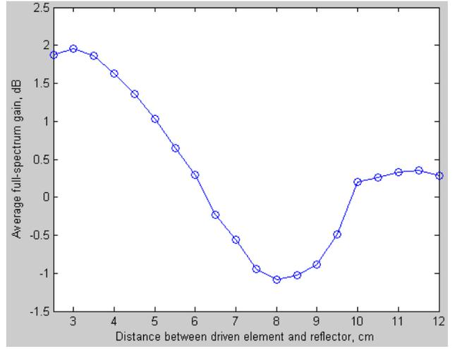
Fig. 5. Results of First Element Separation Variation Experiment
